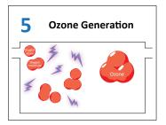
Because of its short life, ozone is generated on-site. Oxygen atoms and molecules are bonded using an electric field to create ozone.
