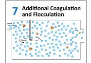
Coagulants are again added to the water, causing impurities to stick together for easier removal (see step 1).
