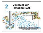
DAF systems introduce micron-sized bubbles that attach to the floc and rise to the surface. This floating bed of particles is removed by a skimmer.
