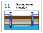
Finished, treated water is injected into the groundwater aquifer, where further natural treatment occurs before extraction.
