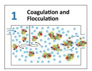
Safe, chemical coagulants are added, causing particles to stick together (floc) and form larger particles, which are more easily removed by subsequent treatment steps.
